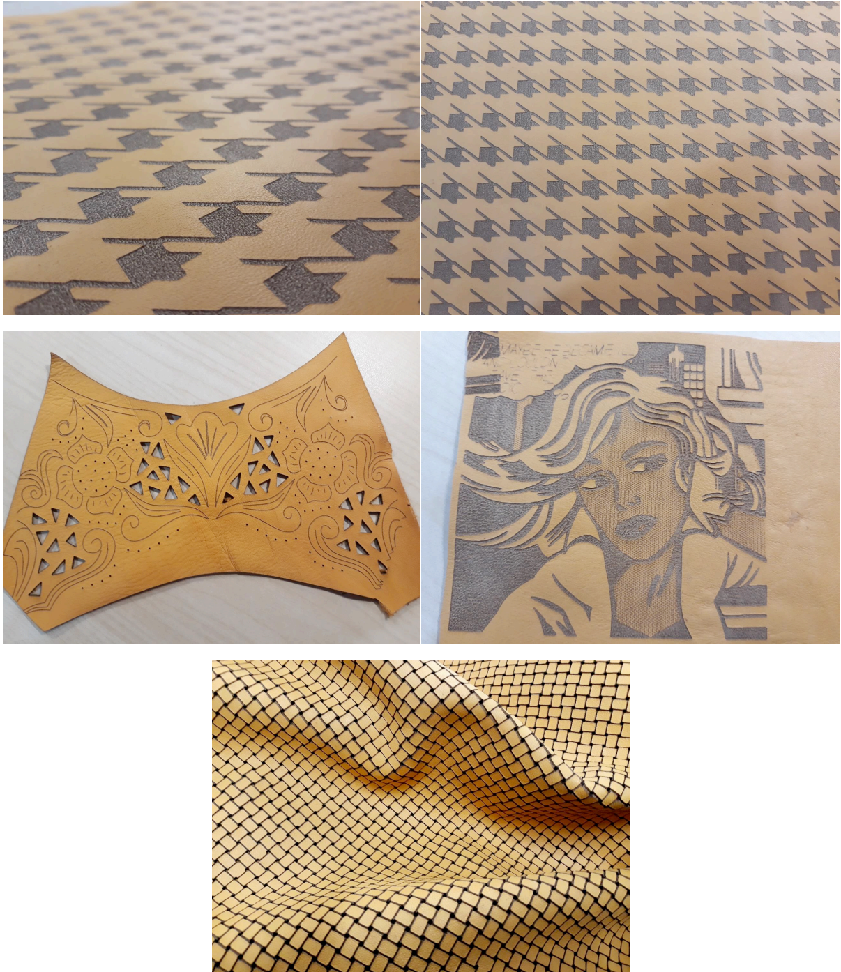
Figure 5: laser marking on leather.
