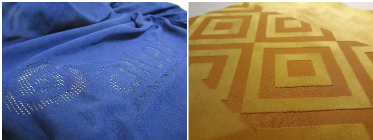
Figure 3: laser marking on synthetic fibres
