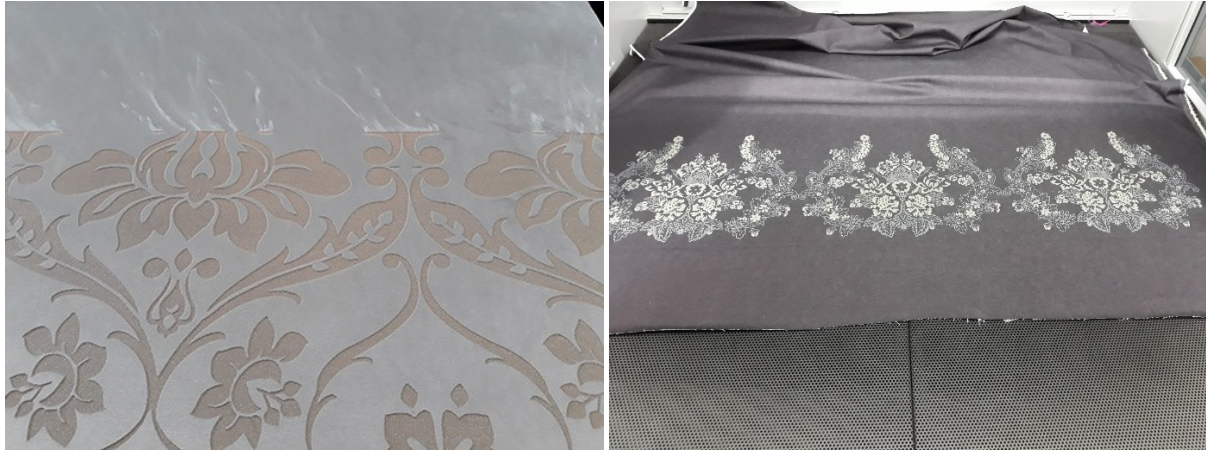
Figure 2: laser marking on cellulosic fibres
