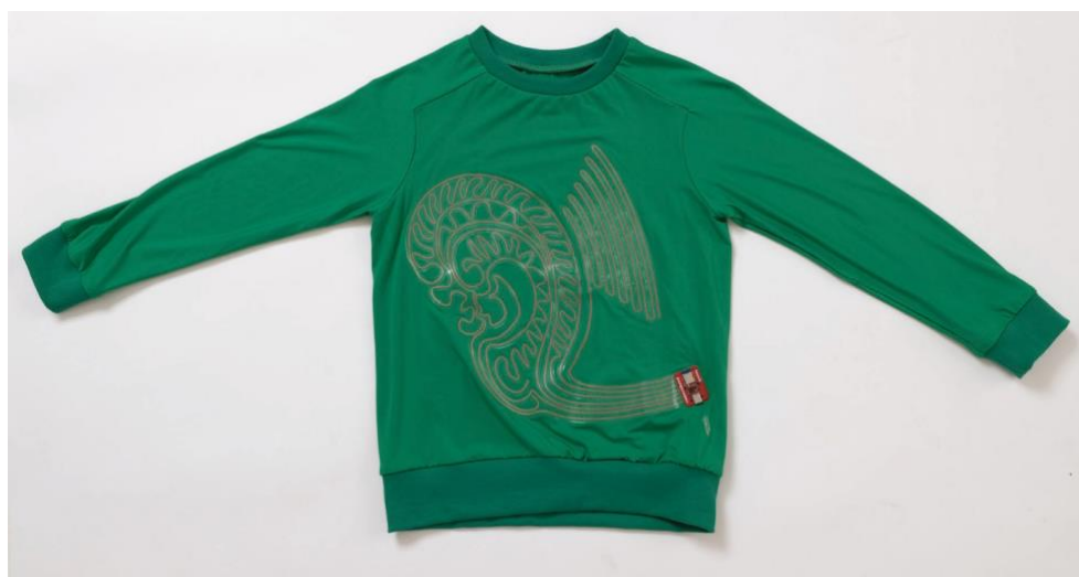
Fig. 14: Touch-sensitive demonstrator realized in TexPCB technology and laminated onto a children's sweater.
