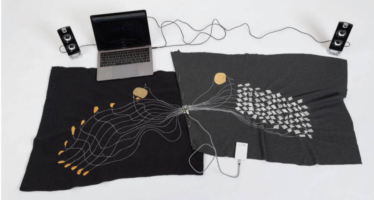
Fig. 10: Embroidered touch sensitive test setup.
