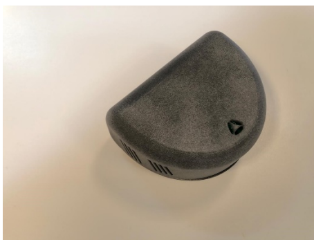
Fig. 3: The pneumatic controller box.
