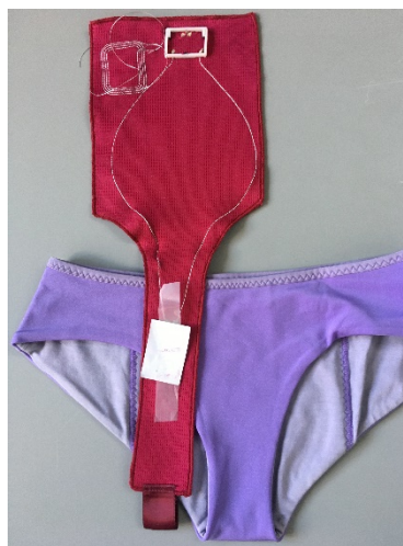
Fig. 10: Alma with embroidered antenna for energy harvesting.
