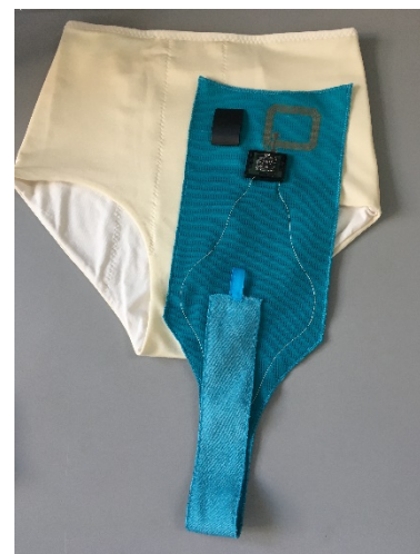
Fig. 11: Alma with laminated 2-layer TexPCB antenna.
