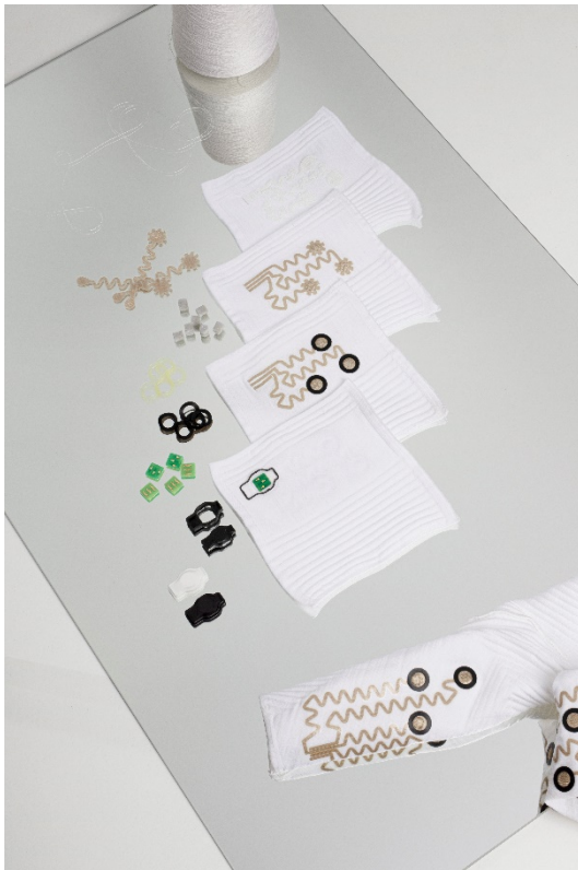
Fig. 5: Textile tracks, sensor, substrate and electronic module for measuring EMG data.
