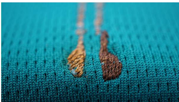
Fig. 12: Textile pH-sensor made of an embroidered reference electrode (left) and working electrode (right).
