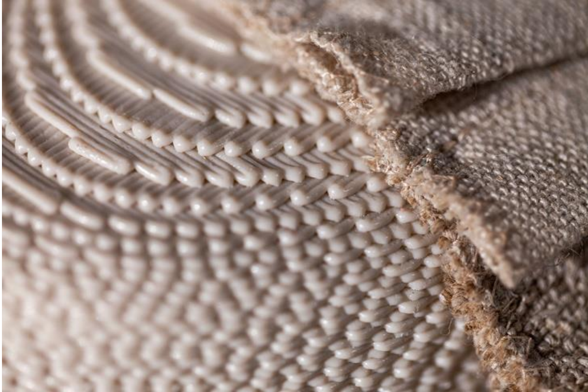
Figure 14: Close-up view of unfilled 3D printed parts and woven upper.
