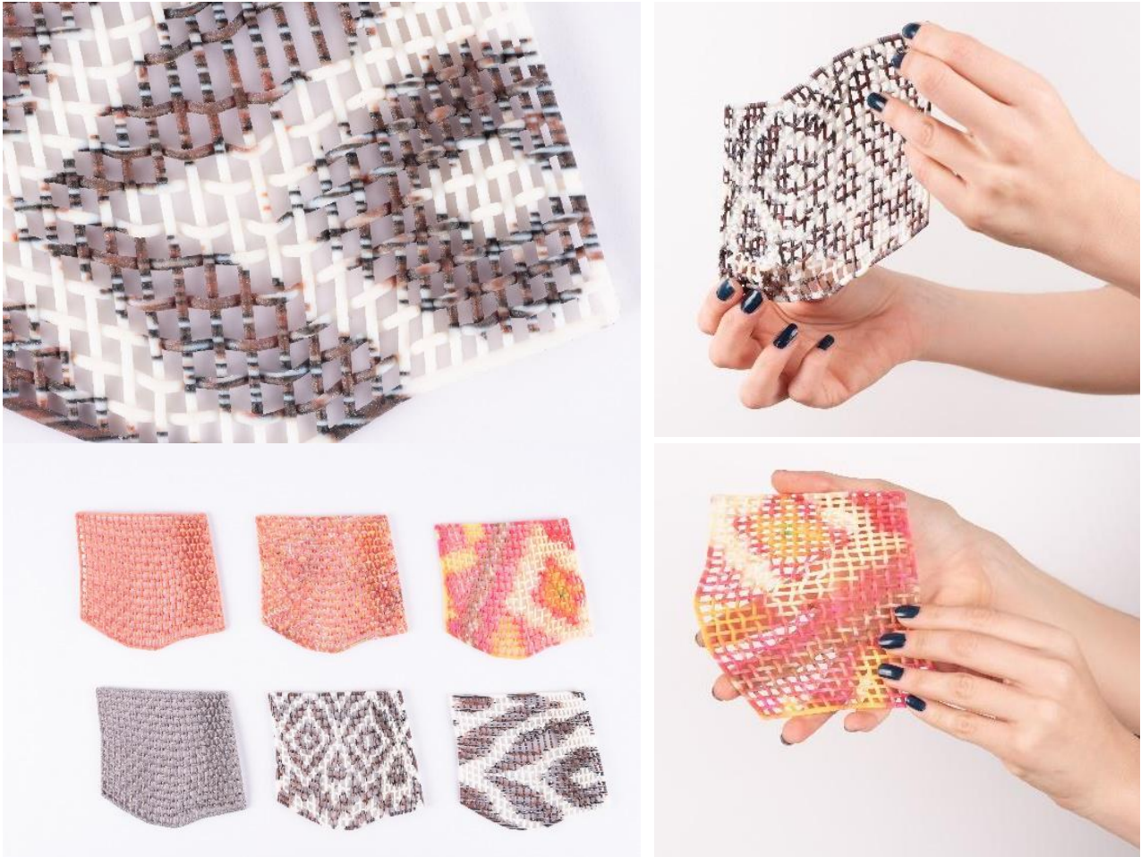
Figure 3 Different printed fiber colors represent different physical properties of flexibility and stiffness. One imitating wool properties and one representing the polymeric fiber.
