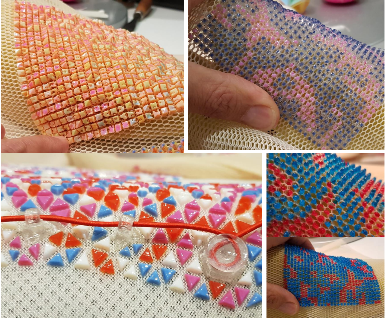
Figure 26: different printed geometries printed on selected fabrics.
