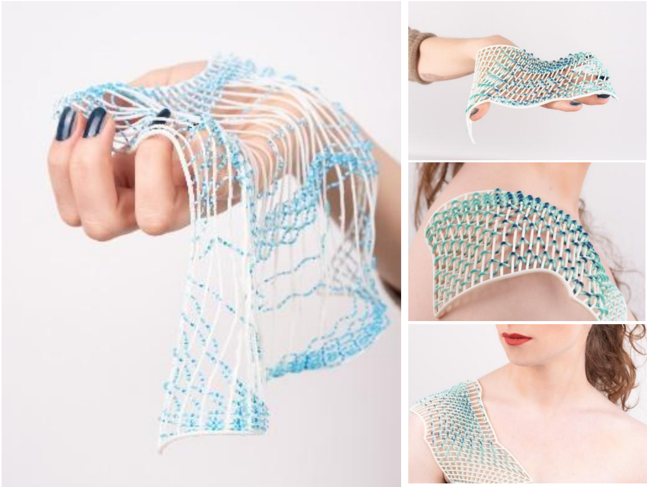
Figure 4 Ganit inserted cotton threads woven inserted in the 3d print
